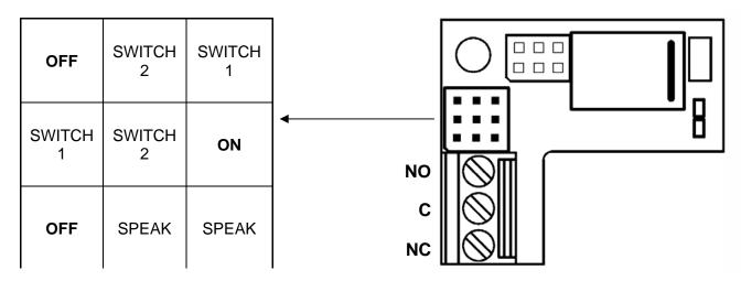
The switch input is available both normally open (between clips **NO** and **C**) as well as normally closed contact (between clips **C** and **NC**).
