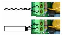
shield to the - terminal. If you use a UTP cable, connect the video signal to such two conductors that are twisted together (making a twisted pair), never use two arbitrary conductors. By connecting or disconnecting the jumper set the impedance match of the video output for the coax cable or twisted pair.
