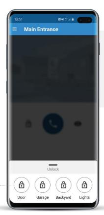
2N® Mobile Video allows you not only to open the selected door, but also to **activate other switches** (please contact your administrator to enable this functionality). You can turn on the lights or trigger an alarm from your mobile phone.
