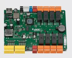
> 8 I/Os with supervised inputs and configurable levels
