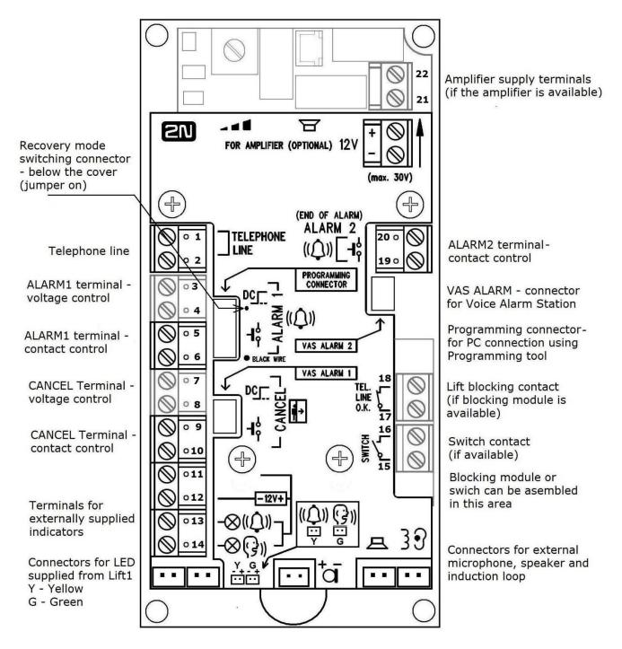
Plugs and connectors on the bottom side of Lift1
