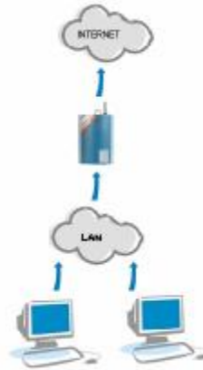
Fig. 61 – Connection of the local LAN network into Internet by means of GPRS
