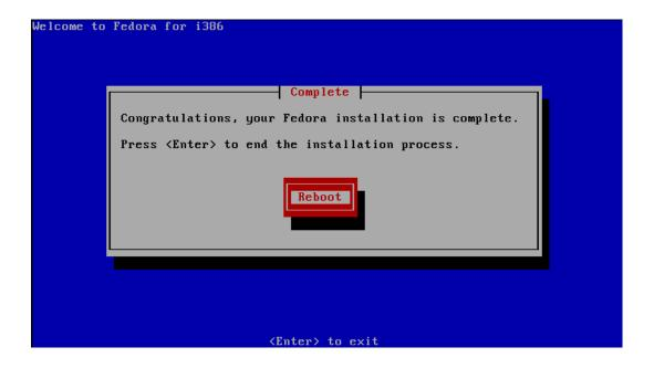
The automatic installation of all the system components takes about 30 minutes (according to the communication HW configuration). After installation, the installator awaits the system **Reboot** confirmation. Press to continue and then remove the CD from the drive. Now you have installed the Linux 32bit OS and associated 2N<sup>®</sup> SIM Star Server installation scripts and packages. Upon the system start, you will be invited to enter the login data.
